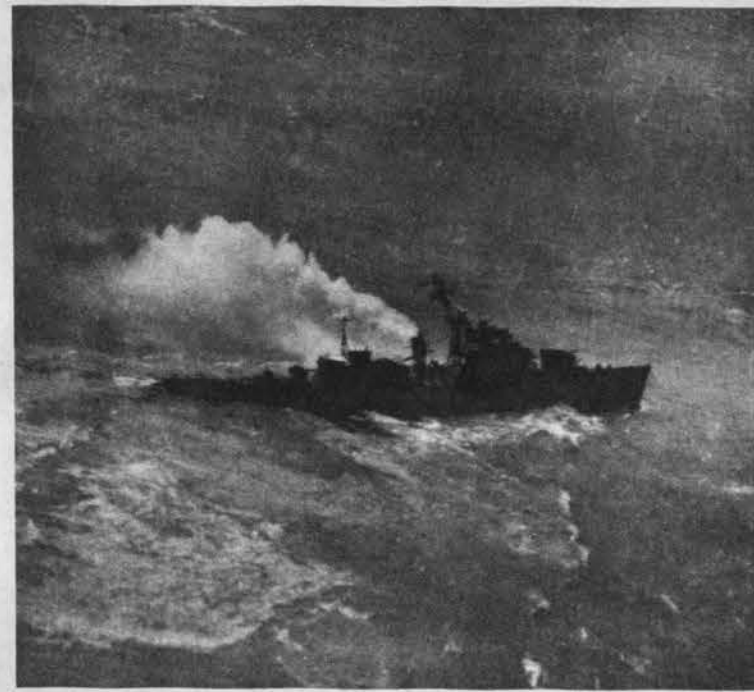
Stack forward and 40 ft. more length distinguish Kaibokan 2 (above) from Kaibokan 1. Otherwise, the two classes are very similar in design.
